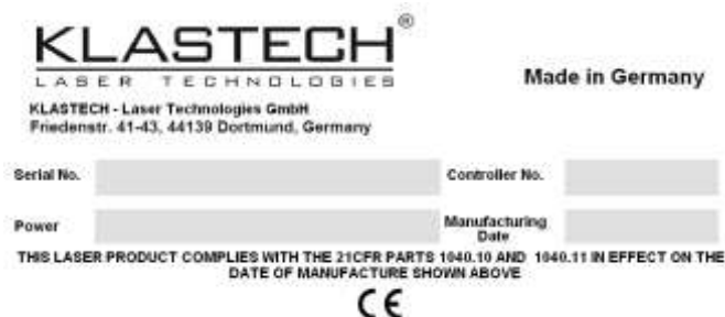
Pic. 1: Sticker located on the laser head and the controller indicating the serial number of the laser and the serial number of the controller.
