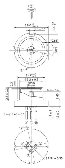
Note: 1. The beam has 12 deg offset against the package reference plane. Please take account it mounted on a board.
