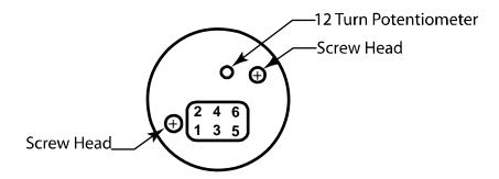
The input connector is inserted with the large Red and Black wires to the left (with the adjustment hole above). If inserted reversed, no damage will result, but the unit will not operate.
