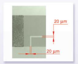
Resistor trimming is performed with ML5 laser machine (*Lasers & Apparatus TM*) using TECH-527 laser.
